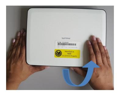
Lift the cover up, while holding the base.
